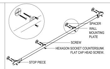
Step 1: Dismount derailing stop from the roller hanger, and screw the roller hanger to the door top as requested location.
